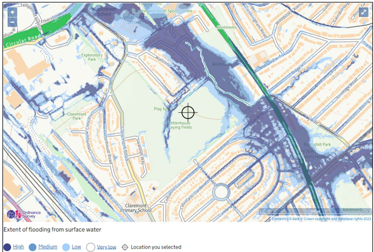
Figure 17: Extent of surface water flooding affecting the Application Site with 'High' representing a greater than 3.3% annual exceedance probability (AEP), 'Medium' representing between 1% to 3.3% AEP, 'Low' representing between 0.1% to 1% AEP, and 'Very Low' less than 0.1% AEP (Environment Agency, 2023).
